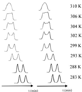
**Figure 2.** Experimental D-HPLC chromatograms of complex **6** (left) in the temperature range of 283–310 K at a constant flow rate using a  $\mu$ -Porasil silica column (particle size 10  $\mu$ m, 30 cm  $\times$  4 mm (inner diameter)) and UV detector at 270 nm, and simulated chromatograms (right):  $N_A = N_B = 8000 \pm 500$ ;  $C_B^0/C_A^0 = 1.30$ , assuming that  $\epsilon_B/\epsilon_A = 1.0$ , and the parameters given in Table 1.
