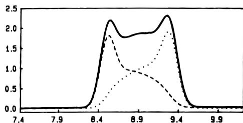
**Figure 1.** An example of a simulated chromatogram showing the curve (solid line) resulting from the sum of the two ideal individual chromatographic curves for injections of pure isomer A (dashed line) or B (dotted line).
